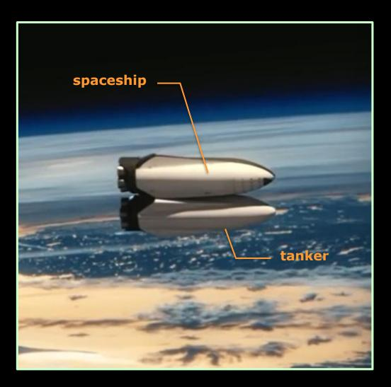
Refueling in Earth orbit before spaceship heads to Mars
