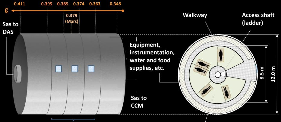
Passengers decks (central one reinforced as radiation shelter)
